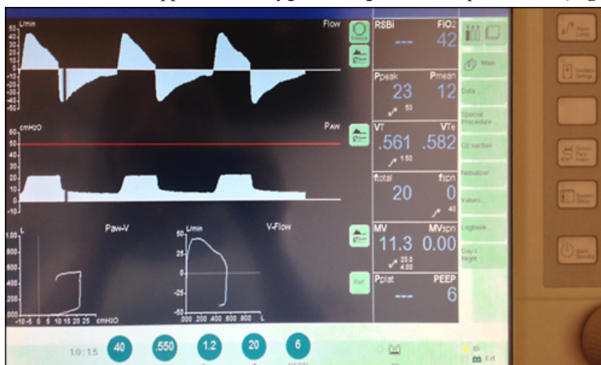
Figure 2: The screen of a ventilator should provide the following minimum information regarding the mode, oxygen concentration (FiO 2 ), flow rate (liters per minute), and programed respiratory rate. Copyright© 2014, EBSCO Information Services.
