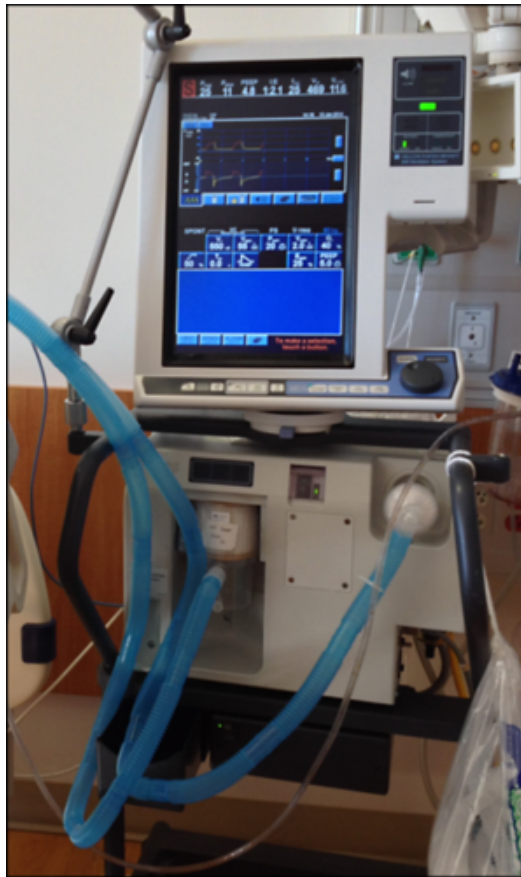
Figure 1: The bedside mechanical ventilator can assist or replace spontaneous breathing. Copyright© 2014, EBSCO Information Services.
